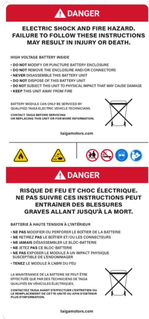
Figure 23: Danger - High Voltage Battery Inside - Orca Carbon
