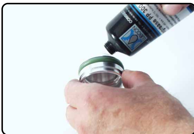
Grease the O-ring with T158.
