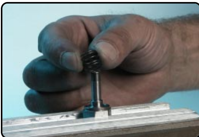
Remove spring check-valve.
