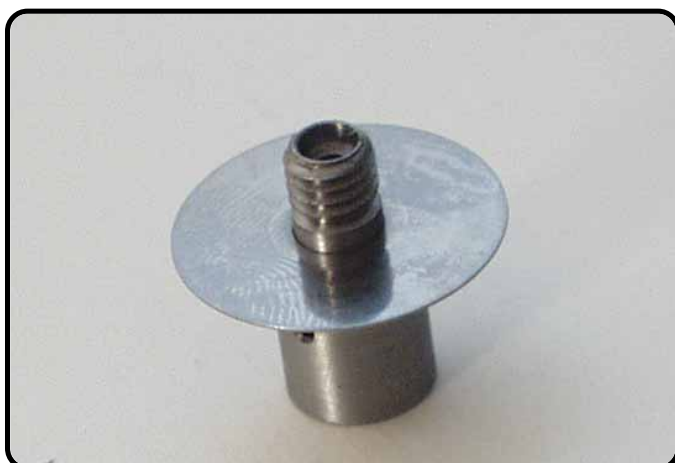
Damping holder with shims (setting).
