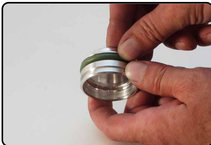
Assemble the O-ring.
