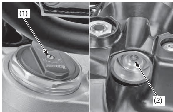
(1) compression damping adjuster (2) rebound damping adjuster
