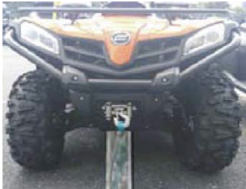
TYPICAL FROUT UP POINT LOCATION
