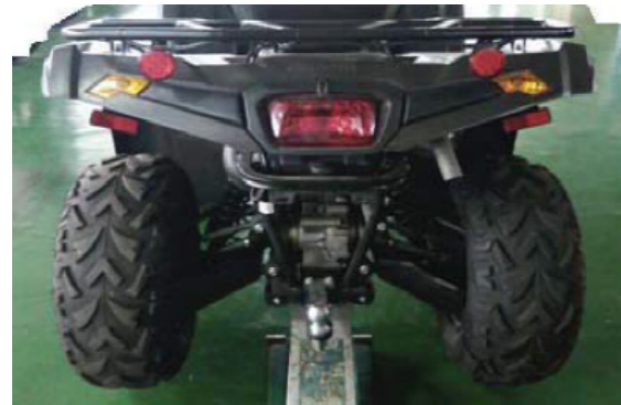
TYPICAL BACK UP POINT LOCATION
