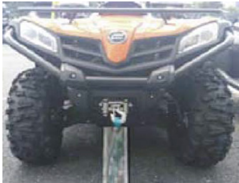
TYPICAL FROUT UP POINT LOCATION
